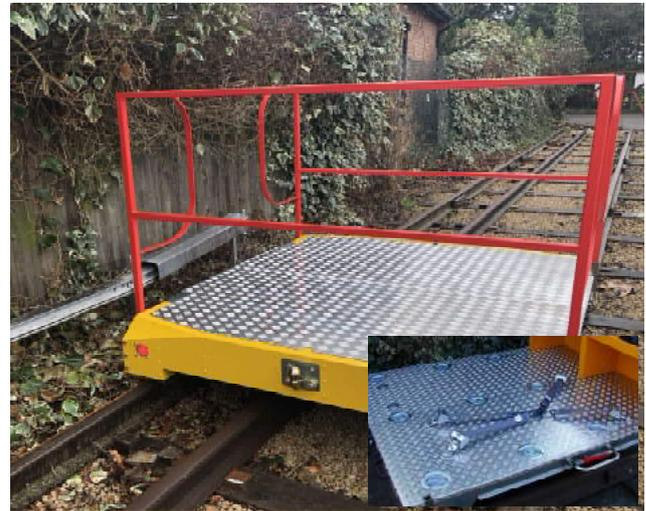
With the addition of bespoke and standard railings the MEP can be turned into an "Emergency Response Vehicle" The umbilical controller now clips to the railings where ever the nominated driver is standing. The unit can be used by emergency responders in full protection suits and BA equipment to get them to site of emergency quickly. The deck comes with evac chair and stretcher securing systems as an option.
