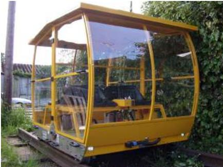
Various roof options are available whether it's a canopy to keep the sun out, roll down pvc windows for hostile weather or full enclosed cabin for DCL can manufacture a bespoke system. All units are removable and foldable for easy storage and transportation
